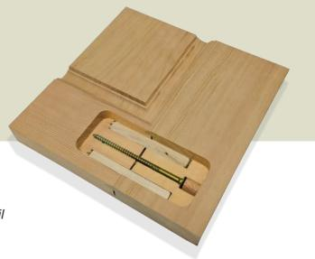
Rogue Premium Plus Doors are assembled with our standard 5/8" x 5" hardwood dowel pins. Then, for added strength and protection to the top and bottom rail joints, we apply additional glue and secure those joints with a 3/8" x 6" steel lag bolt.
